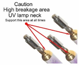
Lamps are shipped clean and sealed in plastic. If accidentally touched, lamp must be wiped with alcohol or Windex before placing in service. Fingerprint contact with the quartz envelope must be avoided. A single fingerprint will etch the quartz surface eventually causing premature failure that will not be covered under warranty.
