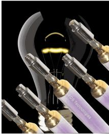
UV lamp (bulb) life depends on many factors including number of starts, thermal operating conditions, power rating, additives and proper handling. Simply defined, it is the hours the lamp produces enough UV energy to properly cure the ink within the availableexposure time.
